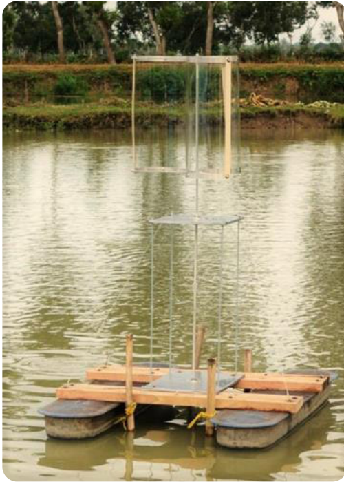
Figure 3.6 Aerator powered by vertical axis wind turbine
