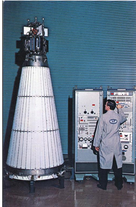
Figure 5: SNAP-10A with its nuclear reactor at the top (Credit: Nuclear Institute)
