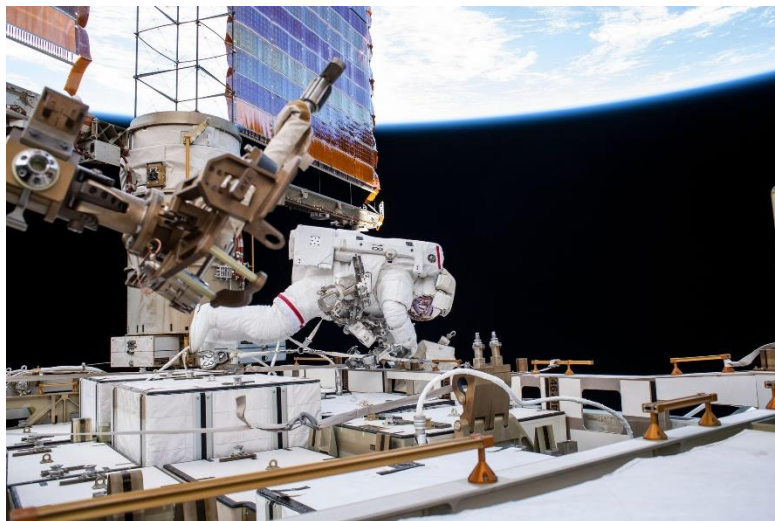
Figure 14: NASA astronaut Andrew Morgan works while tethered on the Port 6 truss segment of the ISS to replace older hydrogen-nickel batteries with the new lithium-ion batteries (Credit: NASA)
