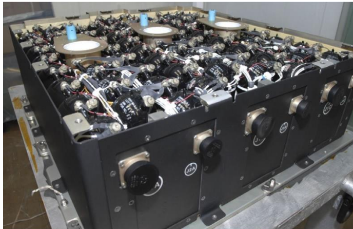
Figure 13: Hubble replacement nickel-hydrogen battery module with the lid removed. Each module weighs 460 pounds and measures 36 inches long, 32 inches wide, and 11 inches high (Credit: NASA)
