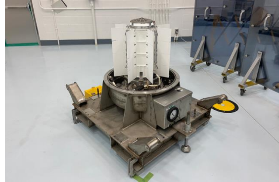
Figure 9: Multi-Mission Radioisotope Thermoelectric Generator (MMRTG) powering the Perseverance Rover (Credit: DOE)
