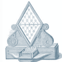
Fig. 150.—Cooke and Wheatstone's Five-Needle Telegraph.
