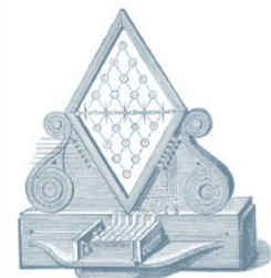
Fig. 750.—Cooke and Wheatstone's Five-Needle Telegraph.
