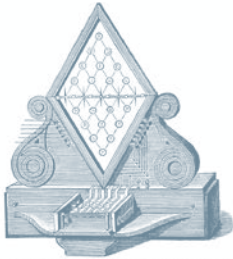
Fig. 750.—Cooke and Wheatstone's Five-Needle Telegraph.
