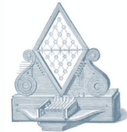
Fig. 750.—Cooke and Wheatstone's Five-Needle Telegraph.
