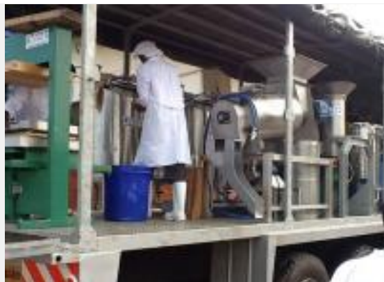
Figure 19: Mobile fruit (juice) processor prototype developed by the FTBIC at Makerere University
