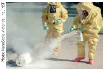
A Kansas emergency response unit tests FAST-ACT on vapors from a leaking propane tank.
