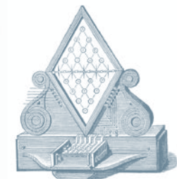
Fig. 750.—Cooke and Wheatstone's Five-Needle Telegraph.
